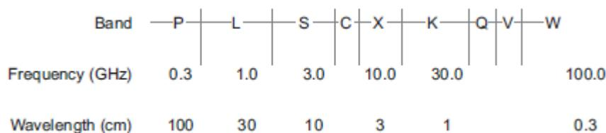
Figure (46): Microwave spectrum and band identification by letters first previous
