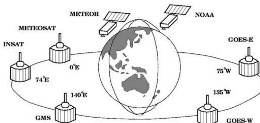
**Figure (5):** Meteorological observation system comprised of geo-stationary and polar satellites.
