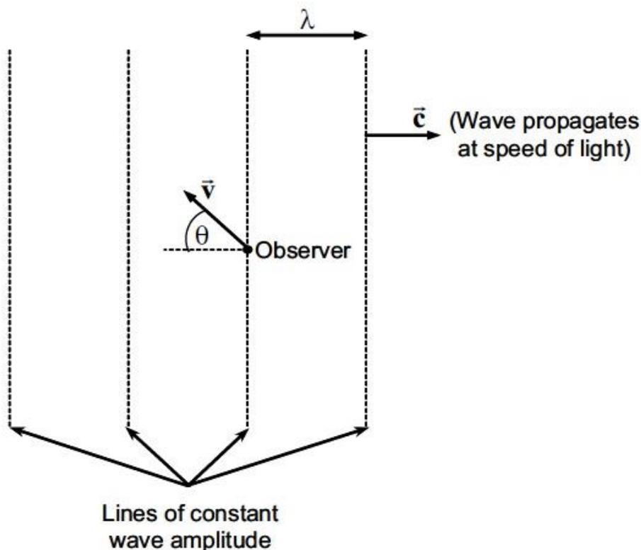
Figure (17): Geometry illustrating wave fronts passing by a moving observer.
