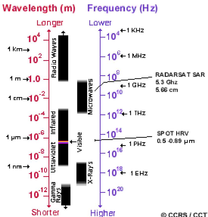
Figure (8): The Electromagnetic Spectrum.
