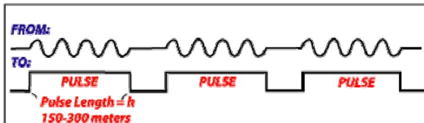
Figure (41): Radar Pulses.
