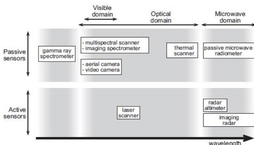
**Figure (4):** Overview of the sensors that are introduced in this section.
