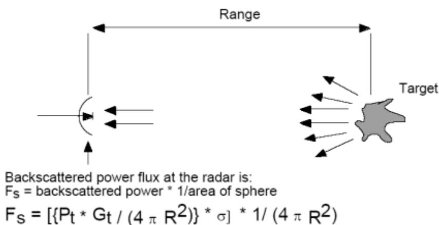
Figure (38): Flux Back Scattered from Target at Radar.
