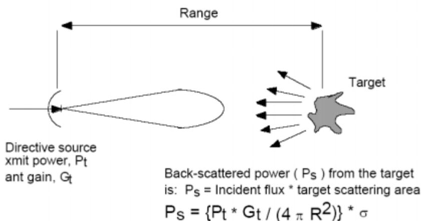
Figure (37): Power Back Scattered from Target with Cross Section.
