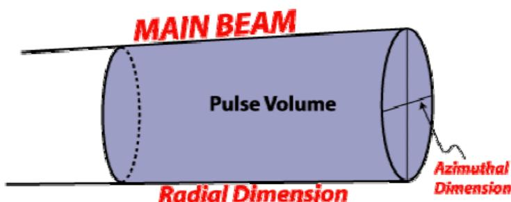
Figure (42): Radar Main Beam and Pulse Volume.
