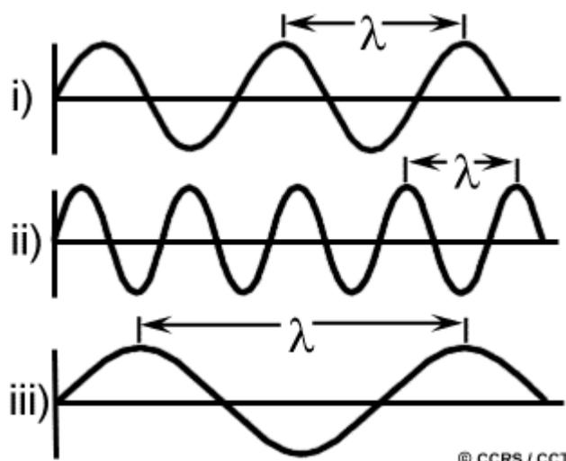
Figure (7): wavelength and frequency.
