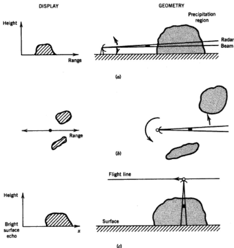
Figure (48): Three rain radar configurations. (a) Range height indicator, (b) plan position indicator, and (c) down looking profile.
