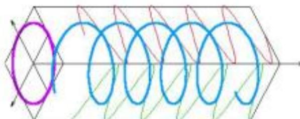
**Figure 11: Circular Polarization.**
