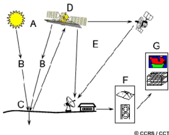
*Figure (1): process of Remote Sensing.*
