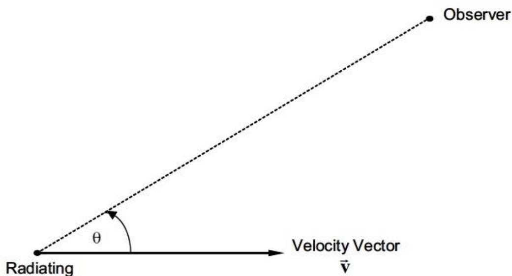
**Figure (16):** Doppler geometry for a moving source, fixed observer.
