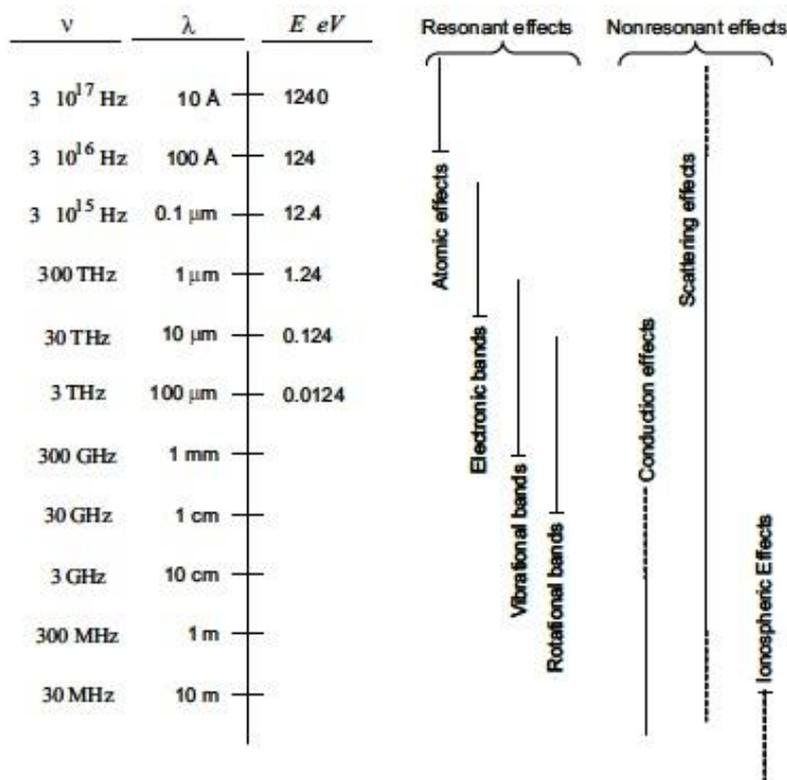
**Figure (21).** Correspondence of spectral bands, photon energy, and range of different wave–matter interaction mechanisms of importance in remote sensing. The photon energy in electron volts is given by  $E(\text{eV}) = 1.24/\lambda$ , where  $\lambda$  is in  $\mu\text{m}$ .
