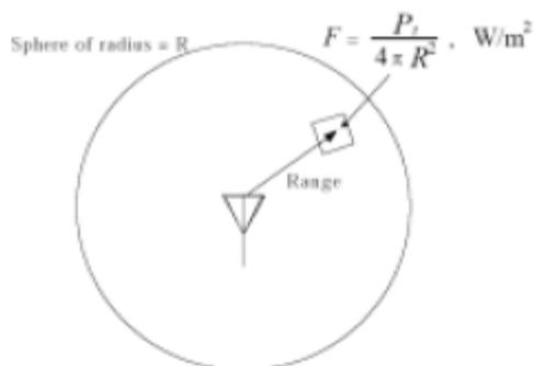
Figure (34): Flux at Distance R
