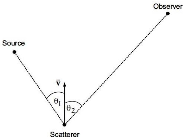
Figure (18): Doppler geometry for a moving scatterer with fixed source and observer.
