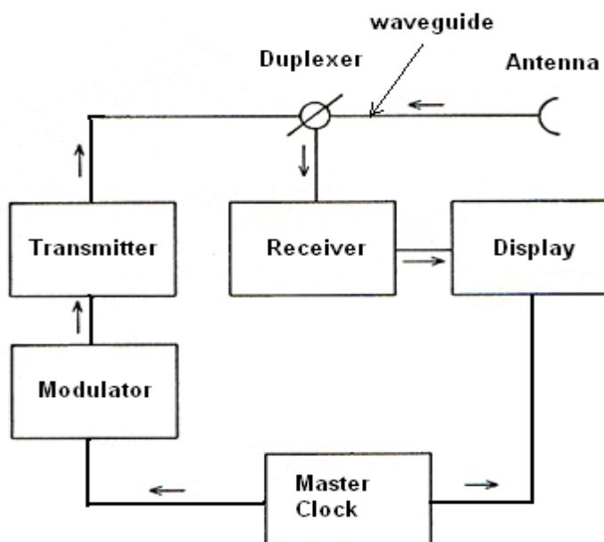
**Figure (45): Basic Radar Diagram.**
