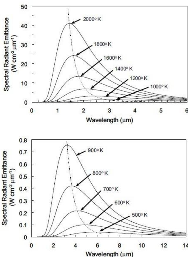
**Figure (20).** Spectral radiant emittance of a blackbody at various temperatures. Note the change of scale between the two graphs.
