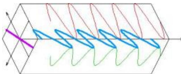
**Figure 10: Linear Polarization.**
