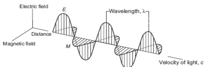
**Figure 47:** A vertically polarized electromagnetic wave; the electric field's Variation occurs in the vertical plane in this example.
