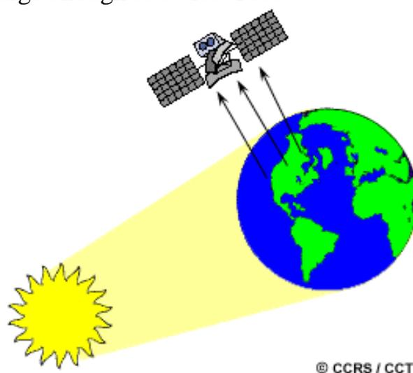
**Figure (2):** Passive remote sensing
