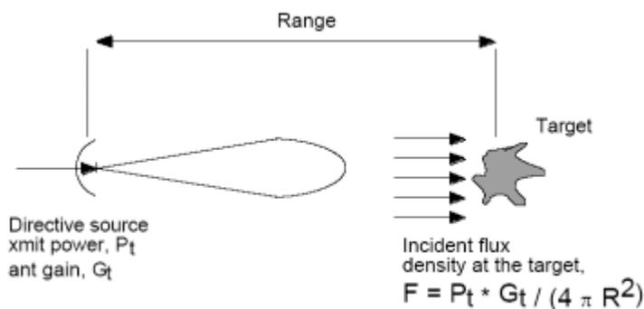
Figure(36): Incident Power Flux Density from a Directive Source.
