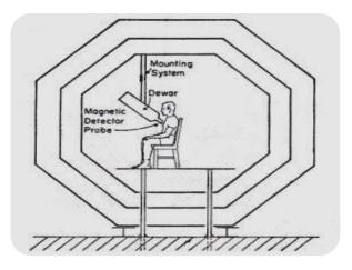
The SQUID magnetometer has also been used to record the magnetic field surrounding the brain. The recording of this field is called the **magnetoencephalogram** or **MEG**. During the alpha rhythm, the magnetic field from the brain is about  $1 \times 10^{-13}$  tesla (T). This is almost one-billionth of the earth's magnetic field.
