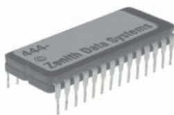
A DIP has two rows of pins that connect the IC circuitry to a circuit board.
