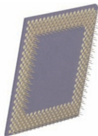
A PGA is a square chip package with pins arranged in concentric squares, typically used for microprocessors.
