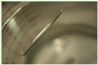
Floating a needle: A carefully placed small needle can be made to float on the surface of water even though it is several times as dense as water. If the surface is agitated to break up the surface tension, then needle will quickly sink.
