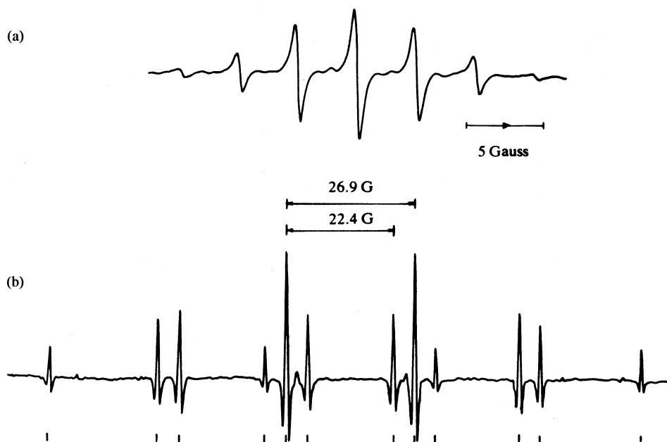
Fig. 12.2. EPR spectra of small organic free radicals. (a) Spectrum of the benzene radical anion. [From J. R. Bolton, Mol. Phys. 6 :219 (1963). Reproduced by permission of Taylor and Francis, Ltd.] (b) Spectrum of the ethyl radical. [From R. W. Fessenden and R. H. Schuler, J. Chem. Phys. 33 :935 (1960); J. Chem. Phys. 39 :2147 (1963). Reproduced by permission of the American Institute of Physics.]
