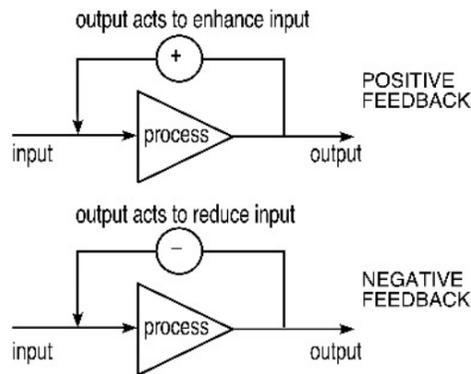
Feedback processes can be classified as positive or negative. In positive feedback a portion of the output is fed back to the input and acts to further stimulate the process. In the case of negative feedback, the portion of the output is subtracted from the input and acts to dampen the process.
