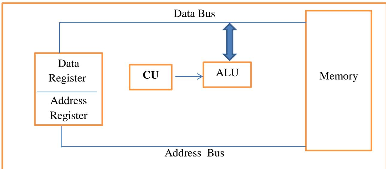
**Figure (2): A Block Diagram of the Simple CPU**
