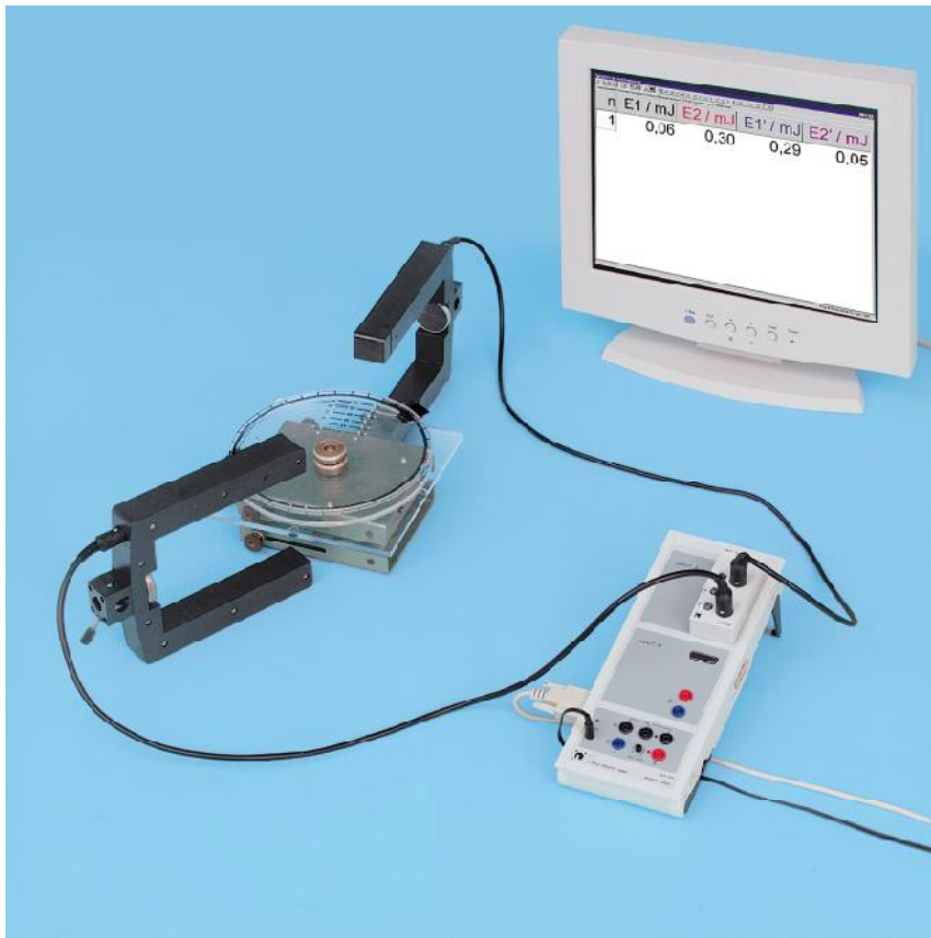
Conservation of angular momentum for elastic torsion impact (P 1.4.2.1)
