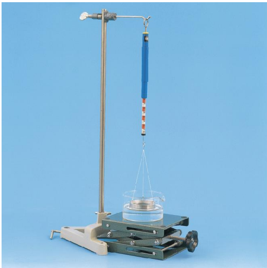
Measuring the surface tension using the tear-away method (P 1.8.4.1)
