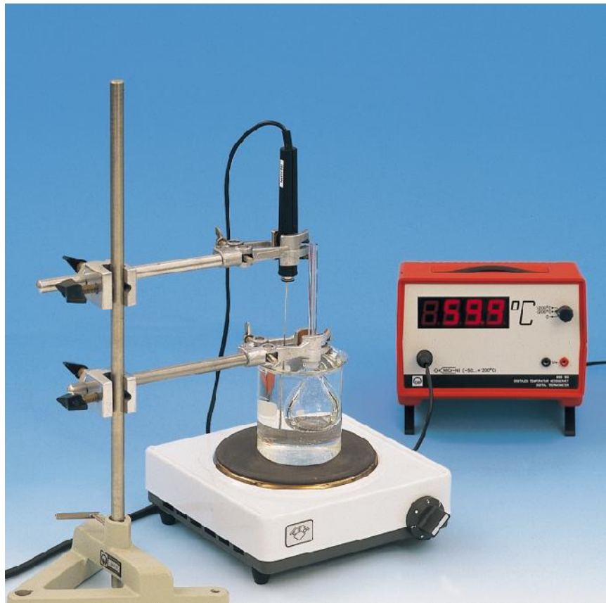
Determining the volumetric expansion coefficient of liquids (P 2.1.2.1 b)
