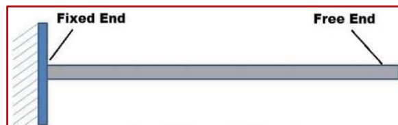
Fig (3) cantilever beams
