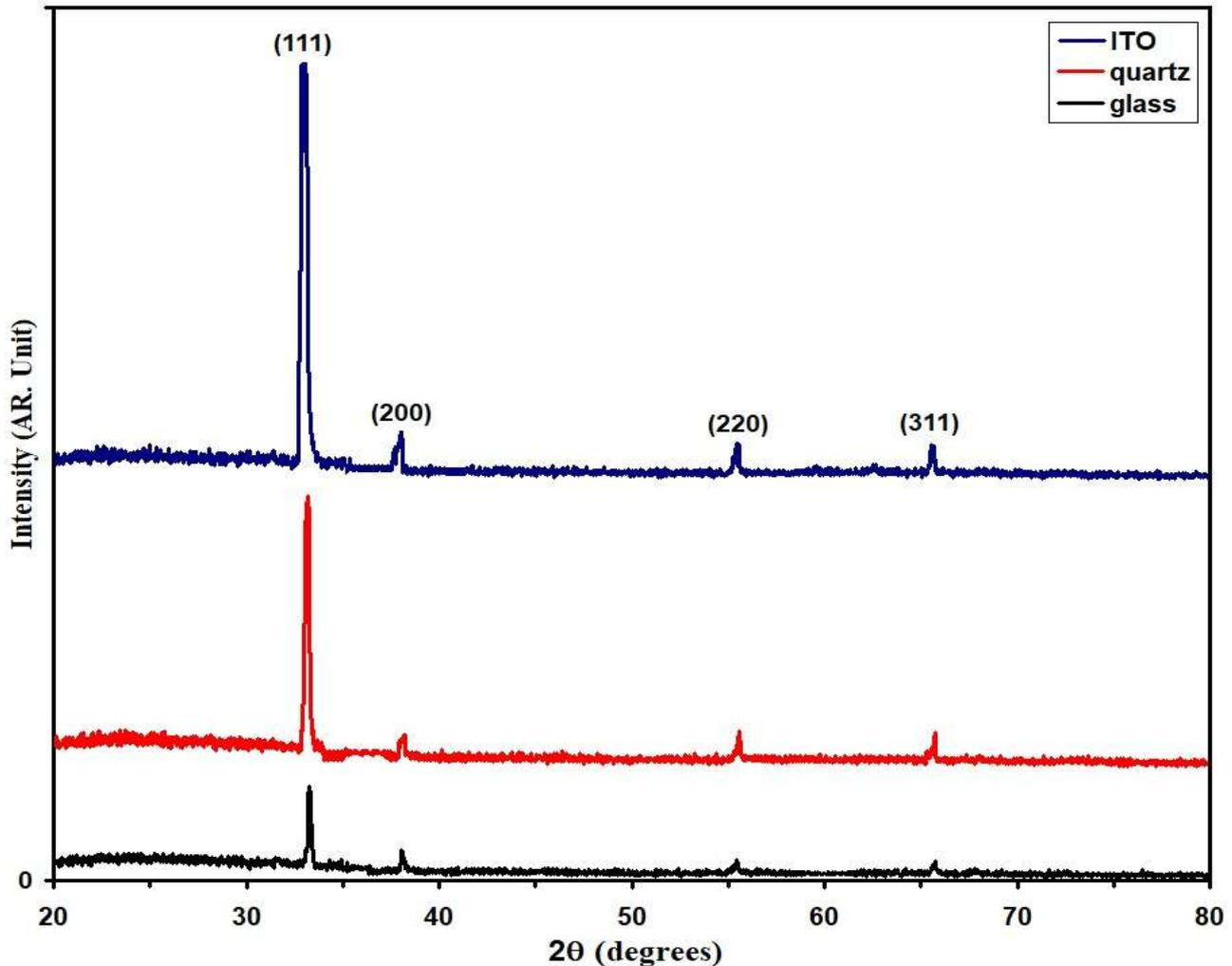
Fig. 1. XRD patterns of deposited films on various substrate types
