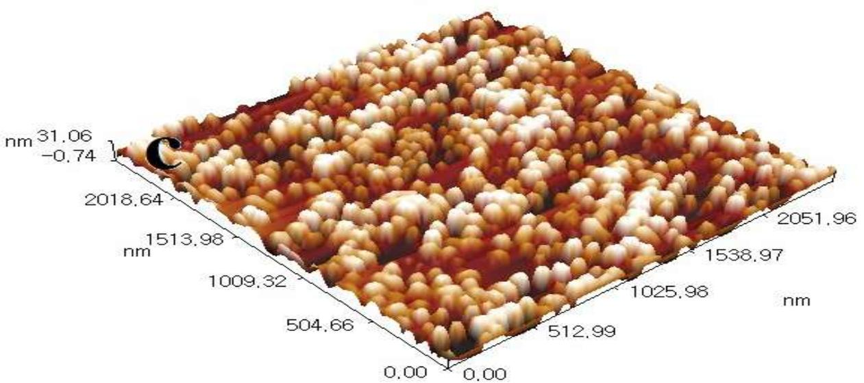
Fig. 4. AFM images and Granularity distributed curve (ITO)
