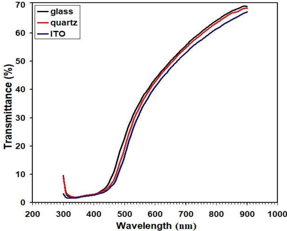
Fig. 5. Transmittance spectra of CdO films grown on various substrate types
