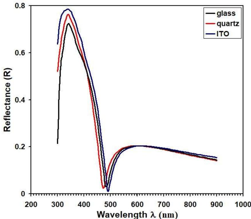
Fig. 6. Reflectance spectra of CdO films grown on various substrate types.
