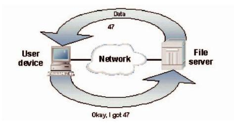
Layer 5, the session layer, provides various services, including tracking the number of bytes that each end of the session has acknowledged receiving from the other end of the session. This session layer allows applications functioning on devices to establish, manage, and terminate a dialog through a network. Session layer functionality includes:
