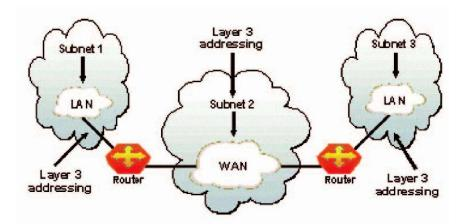
Layer 3, the network layer of the OSI model, provides an end-to-end logical addressing system so that a packet of data can be routed across several layer 2 networks (Ethernet, Token Ring, Frame Relay, etc.). Note that net-work layer addresses can also be referred to as logical addresses.
