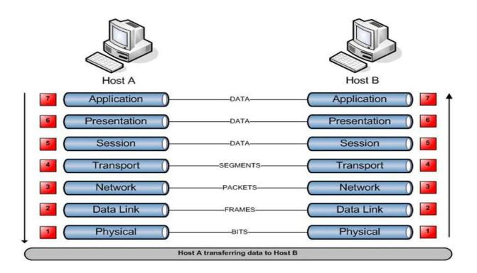
A networking model offers a generic means to separate computer networking functions into multiple layers. Each of these layers relies on the layers below it to provide supporting capabilities and performs support to the layers above it. Such a model of layered functionality is also called a "protocol stack" or "protocol suite".
