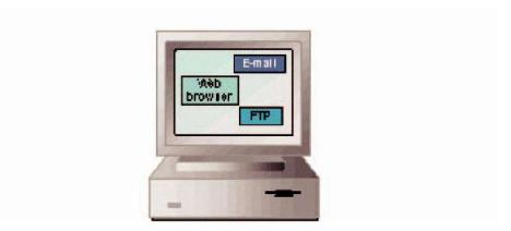
Layer 7, the application layer, provides an interface for the end user operating a device connected to a net-work. This layer is what the user sees, in terms of loading an application (such as Web browser or e-mail); that is, this application layer is the data the user views while using these applications.
