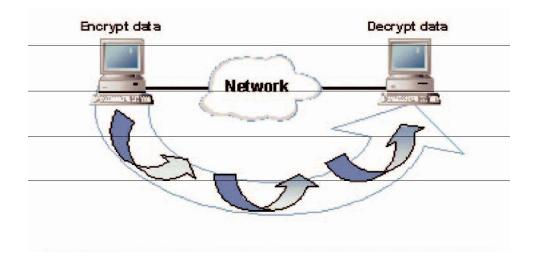
Layer 6, the presentation layer, is responsible for how an application formats the data to be sent out onto the network. The presentation layer basically allows an application to read (or understand) the message. Examples of presentation layer functionality include:
