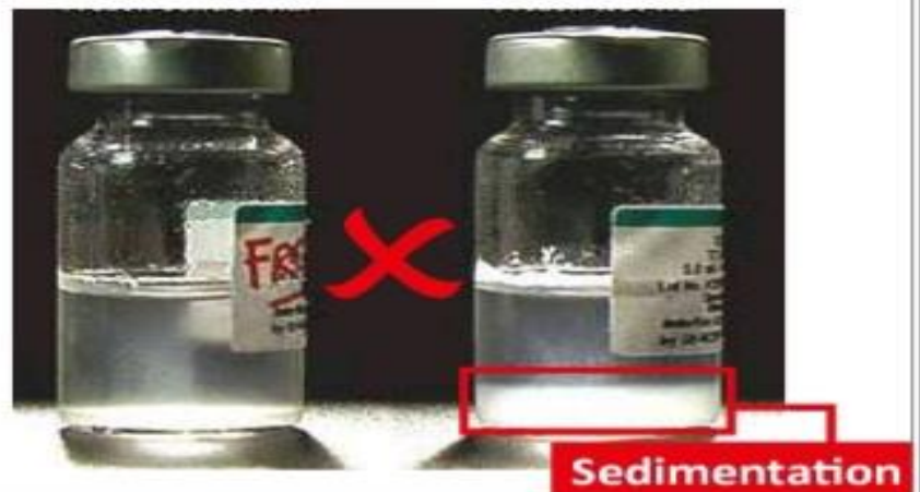
Fig. 4.11: Shake Test Failed - Do not use Vaccine
