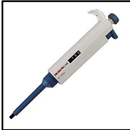
Micropipette ( small volumes measuring device)
