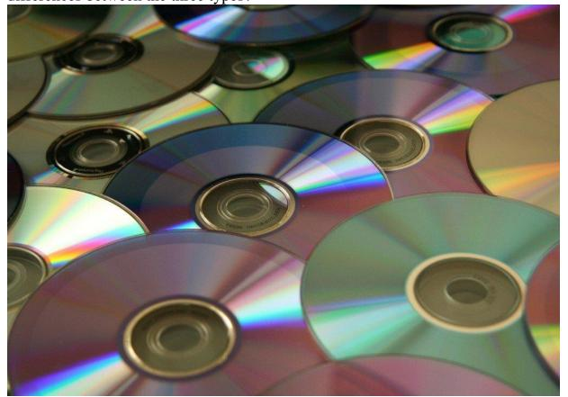
❖ **Digital Versatile Disk (DVD)**: it's similar to CD but with high capacity (17 gigabyte). It used to store high quality films, videos. Both DVDs and CDs look alike in size and shape and are used for the same purpose. Just because they look identical and have the same usage, we cannot conclude that both CDs and DVDs are the same. The following are some of the differences between a CD and a DVD.
