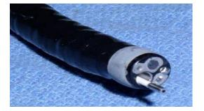
Since light contains energy that largely appears as heat when it is absorbed, there is a limit on the amount of light that can be used in endoscopy. For endoscopy, the heating can be reduced by reducing the IR light from the source with special IR absorbing glass filters. In this cold-light endoscopy the light source contains very little IR radiation and the heating of tissues is minimized.
