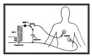
The paddles are metal electrodes **7.5cm** in diameter that are coated with conductive paste and placed **above** and **below** the heart. The paddle handles are made of plastic and are electrically insulated to prevent accidental shock to the operator.
