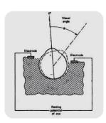
Electrooculograms provide information on the orientation of the eye, its angular velocity, and its angular acceleration.
