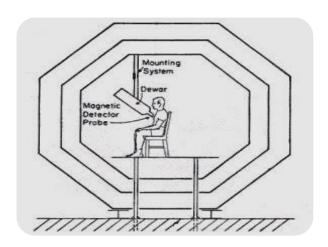
The SQUID magnetometer has also been used to record the magnetic field surrounding the brain. The recording of this field is called the **magnetoencephalogram** or **MEG**. During the alpha rhythm, the magnetic field from the brain is about  $1x10^{-13}$  tesla (T). This is almost one-billionth of the earth's magnetic field.
