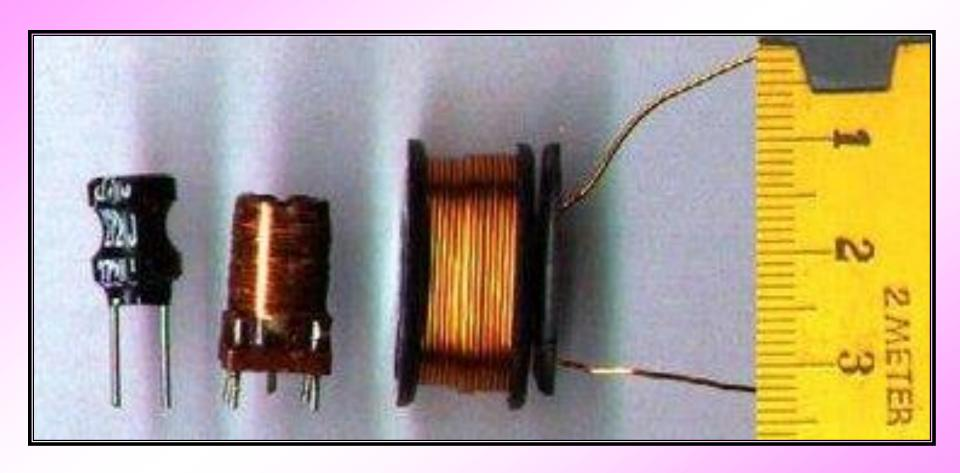
**Inductor** is an electric device consisting of one or more turns of wire and typically having **two** terminals. An **inductor** is usually connected into a circuit in order to raise the **inductance** to a desired value.
