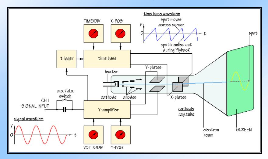
Cathode rays exist in the form of streams of high-speed electrons emitted from the heating of a (**cathode**) inside a vacuum tube, at its rear end. The electron beam emitted by the heated (**cathode**) at the rear end of the tube is accelerated and focused by one or more (**anode**), and strikes the front of the tube, producing a bright spot on the phosphorescent screen.
