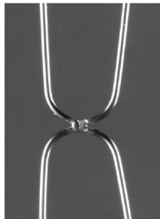
FIGURE 1- Round joints. Wire material: Forestant in spring hard quality (diameter 0.9 mm)
