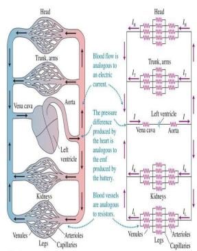
Modeling the human circulatory system as an electric circuit
