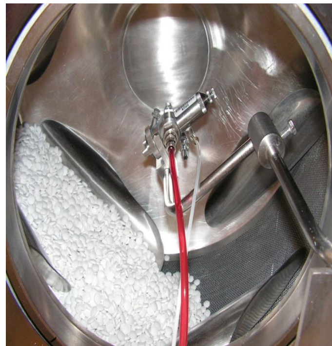
Spraying Wetting Recrystallisation Coated particle
