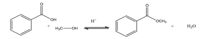
For this experiment, you will isolate the product, methyl benzoate, and any unreacted benzoic acid. Using this data, you will calculate the equilibrium constant for the reaction.
