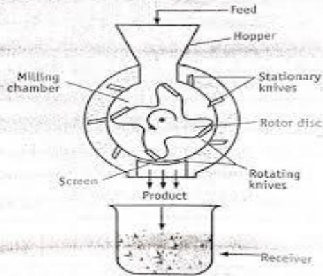
**Cutting mill is used for tough materials , fibrous materials & provide a successive cutting or shearing action rather than attrition or impact.**
