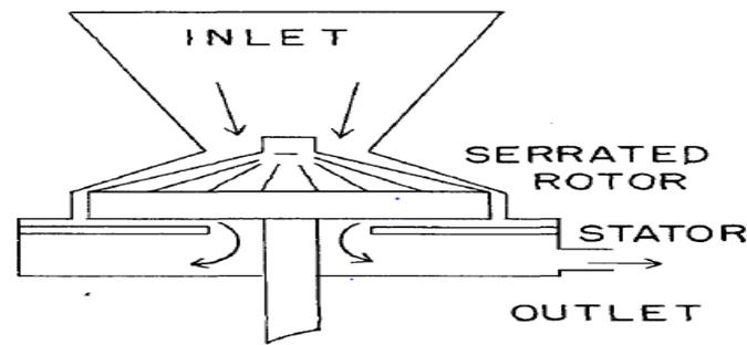
Consists of a high speed rotor & stator with conical milling surfaces between which in is an adjustable clearance .
