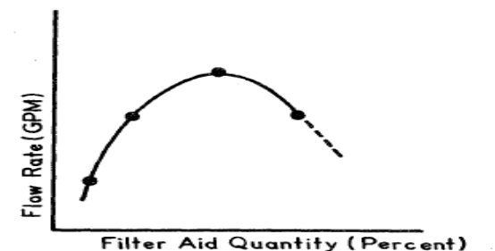
FIG. 7-1. Experimental determination of flow rate as a function of filter aid quantity discloses correct operating level.
