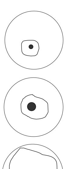
Object seen in low-power field: Approximate length:  $\frac{22}{10x10} * 1000 = 220 \ \mu m$  $\frac{33.5}{100} * 220 = 73.7 \ \mu m$
