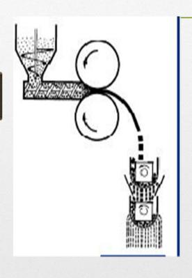
Two rolls rotate against each other, to increase the density of powder by pressing it between the rollers and get a thin wide sheet or ribbon equivalent to the slug produced by slugging, then these ribbons or aggregates are screened to produce uniform granules.
