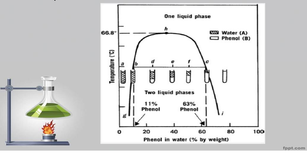
The curve g b h c i shows limits of temperature and encentration within which two liquid phases exist in equilibrium.
