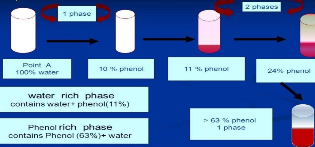
**binodal curve :-** is the curve that separates two phase area from one phase area .
