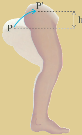
Fig. 7-B The runner's center of mass moves from point P to point P', increasing elevation by a distance h .
