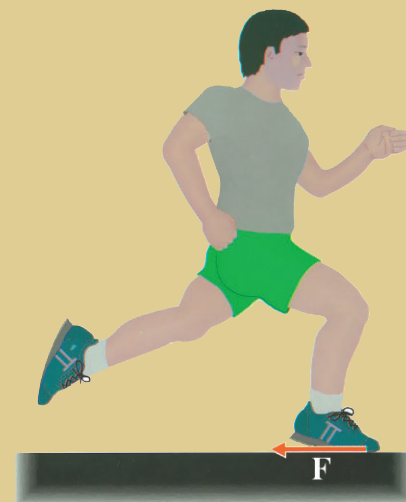
Fig. 7-C The road exerts a backward force on a runner's foot as it hits the surface. This force tends to reduce the runner's speed.
