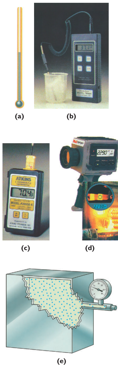
Fig. 12-1 Thermometers. The length of a column of mercury indicates temperature in a mercury thermometer (a) . Electrical properties of a probe are used to measure temperature in a thermistor thermometer (b) and a thermocouple thermometer (c) . In an optical pyrometer (d) , used to measure very high temperatures, light emitted by the hot body is compared with light produced by an electrically heated filament inside the pyrometer. (e) Gas pressure indicates temperature in a constant-volume gas thermometer.
