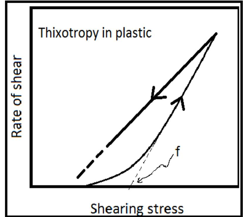
**Rheograms obtained with thixotropic materials are highly dependent on the rate** at which shear is increased or decreased and the **length of time a sample** is subjected to any one rate of shear.
