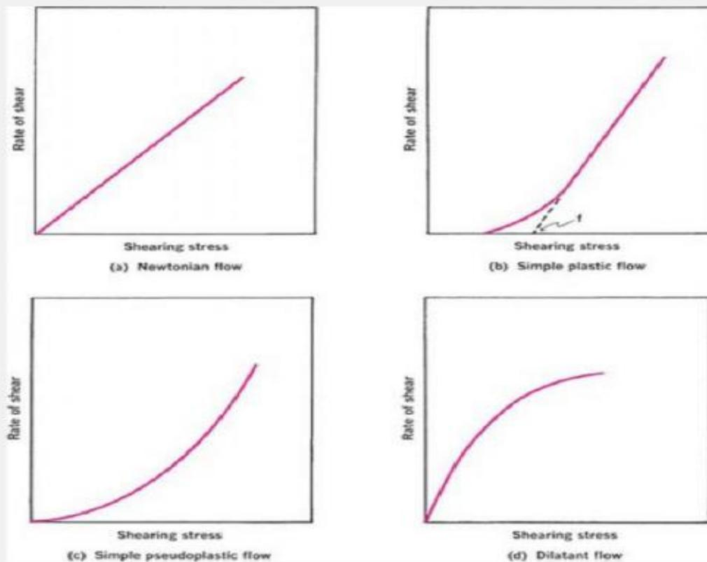
**Fig. 19-2.** Representative flow curves for various materials.
