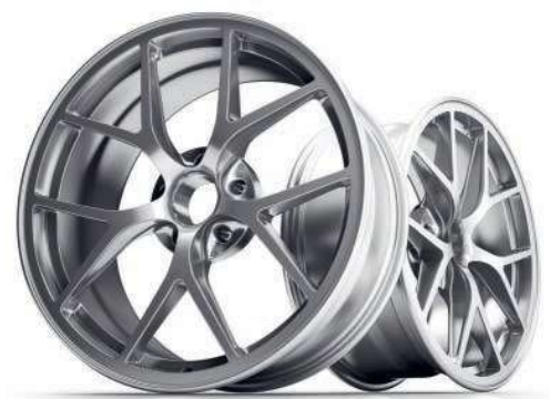
▲ Figure 2.36 Alloy wheel made by 3D printing
