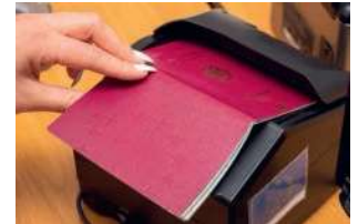
▲ Figure 2.23 Using OCR to process a passport
