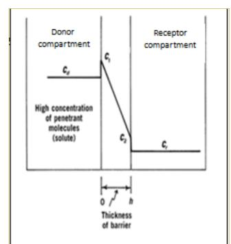
It is normal for the concentration curve to increase or decrease sharply at the boundaries of the barrier because, in general, C1 is different from Cd, and C2 is different from Cr
