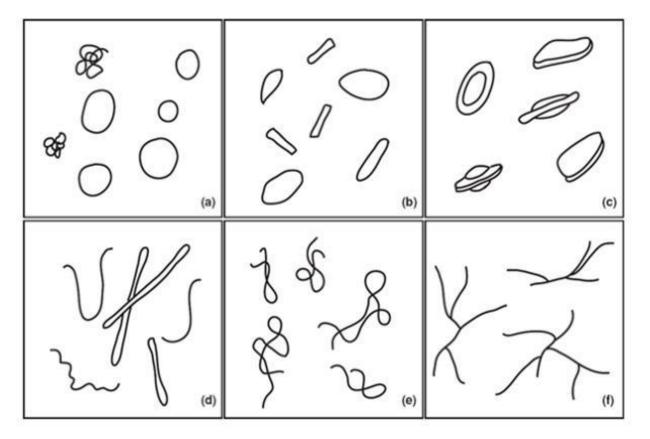
Some shapes that can be assumed by colloidal particles: (a) spheres and globules, (b) short rods and prolate ellipsoids, (c) oblate ellipsoids and flakes, (d) long rods and threads, (e) loosely coiled threads, and (f) branched threads.
