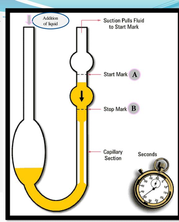
the absolute viscosity of the unknown liquid, $\eta_1$  is determined by substituting the experimental values in the equation:
