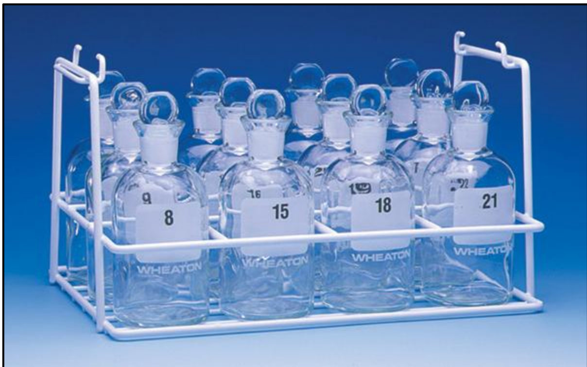
Figure 7.2 a rack of bottles used for measuring the Biochemical Oxygen Demand (BOD)
