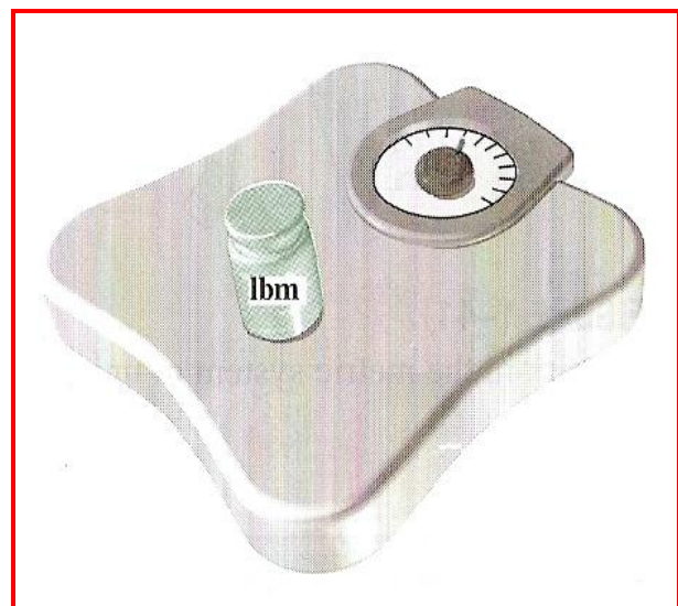
Figure 1-2. A mass of 1 lbm weight 1 lbf on earth.
