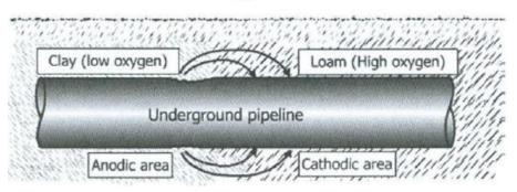
There are three general types of concentration cell corrosion:
