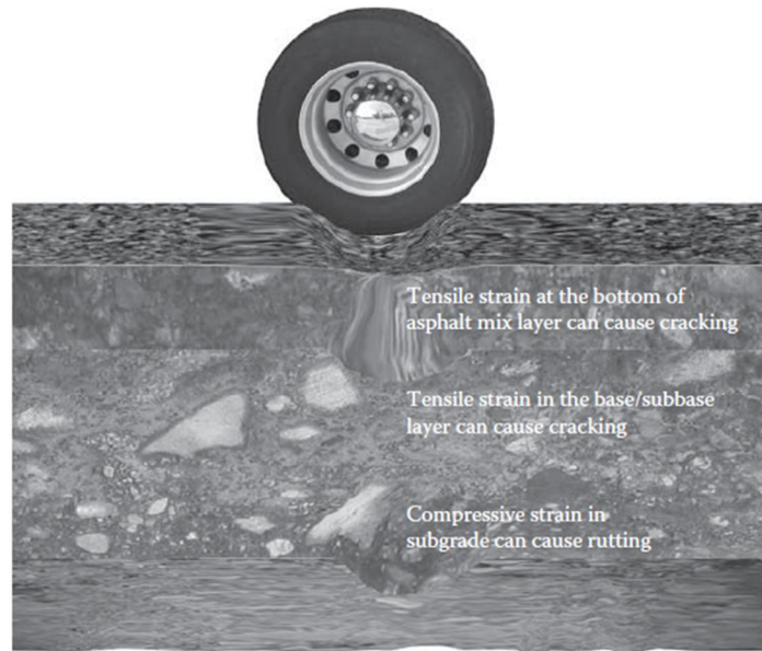
FIGURE 2.6 Major distress-causing responses in a “flexible” or asphalt mix pavement.
