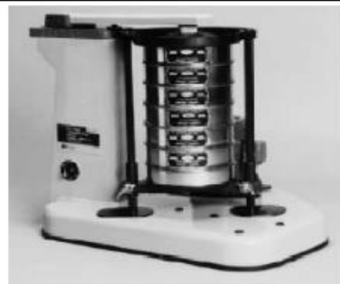
A set of sieves for a test in the laboratory
