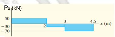
A bronze bar is fastened between a steel bar and an aluminum bar as shown in the Figure. Axial loads are applied at the positions indicated. Find the largest value of P that will not exceed an overall deformation of 3.0 mm, or the following stresses: 140 MPa in the steel, 120 MPa in the bronze, and 80 MPa in the aluminum. Use Est = 200 GPa, Eal = 70 GPa, and Ebr = 83 GPa.
