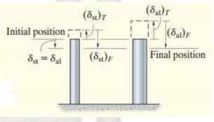
The rigid bar ABC in Figure is pinned at B and attached to the two vertical rods. Initially, the bar is horizontal and the vertical rods are stress-free. Determine the stress in the aluminum rod if the temperature of the steel rod is decreased by 40°C. Neglect the weight of bar ABC.
