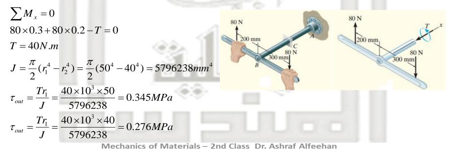
The steel shaft shown below is subjected to two concentrated torques at B and C. If the shear modulus of the steel material G is 80GPa, determine:
