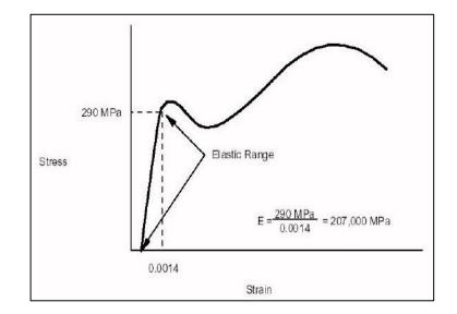
When no straight portion is present in the stress –strain curve, as in the case of concrete material, the Young's modulus can be obtained by one of the following methods.
