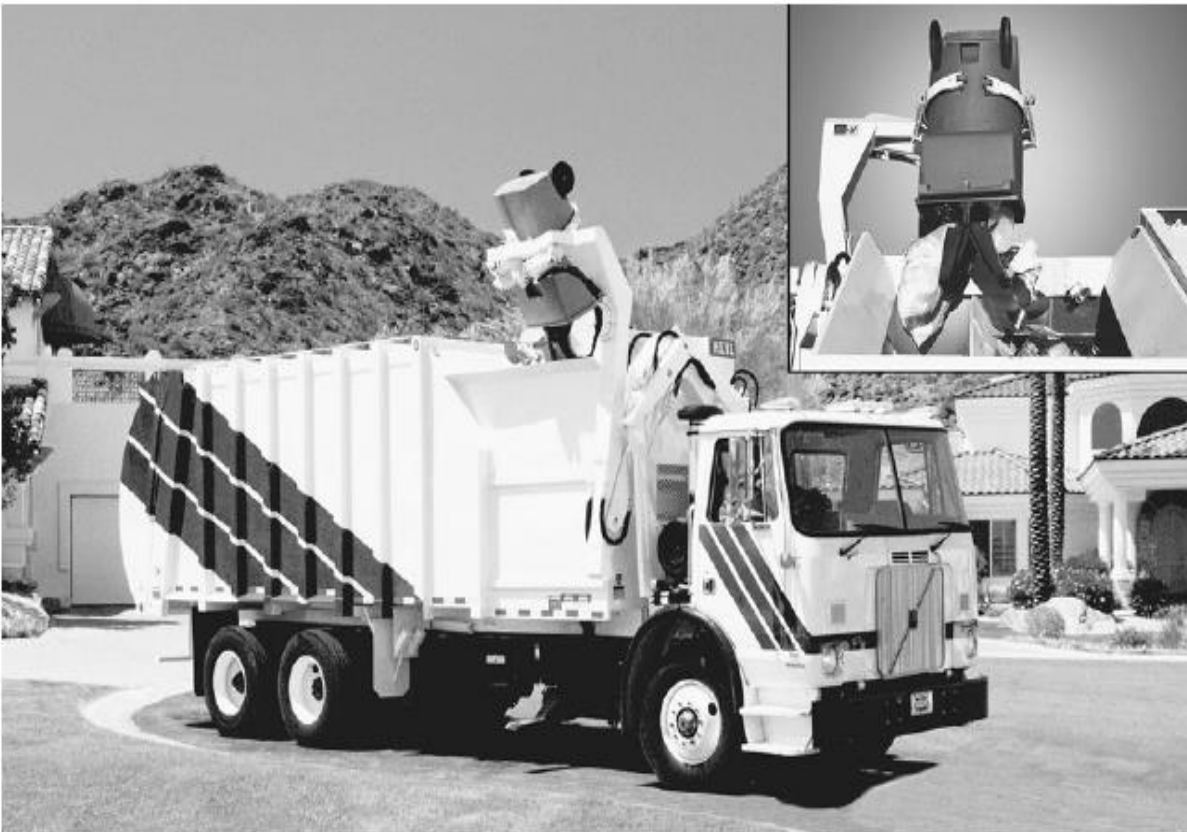
Fig. 2. Typical example of mechanized collection vehicle with mechanical articulated pickup mechanism used for the collection of domestic source waste
