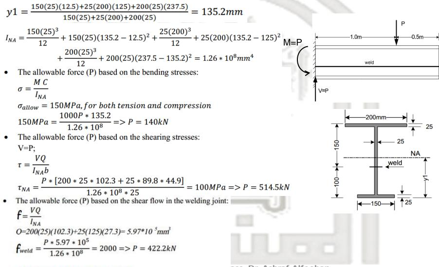
The safe allowable load Psafe = 140kN
