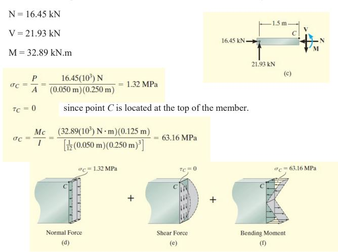
Superposition: The shear stress is zero. Adding the normal stresses determined above gives a compressive stress at *C* having a value of
