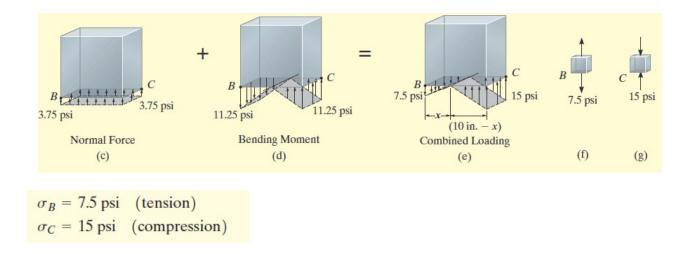
Ex5: The member shown in Fig. has a rectangular cross section. Determine the state of stress that the loading produces at point C.
