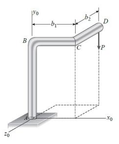
$$b_{1} = 3.6 \text{ ft} \qquad b_{2} = 2.2 \text{ ft} \qquad P = 1400 \text{ lb}$$
