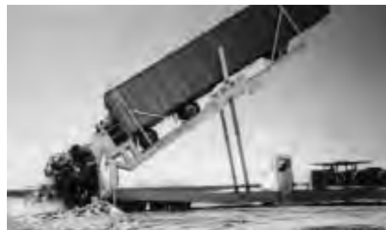
A trailer tipper emptying a transfer trailer at a waste disposal facility.
