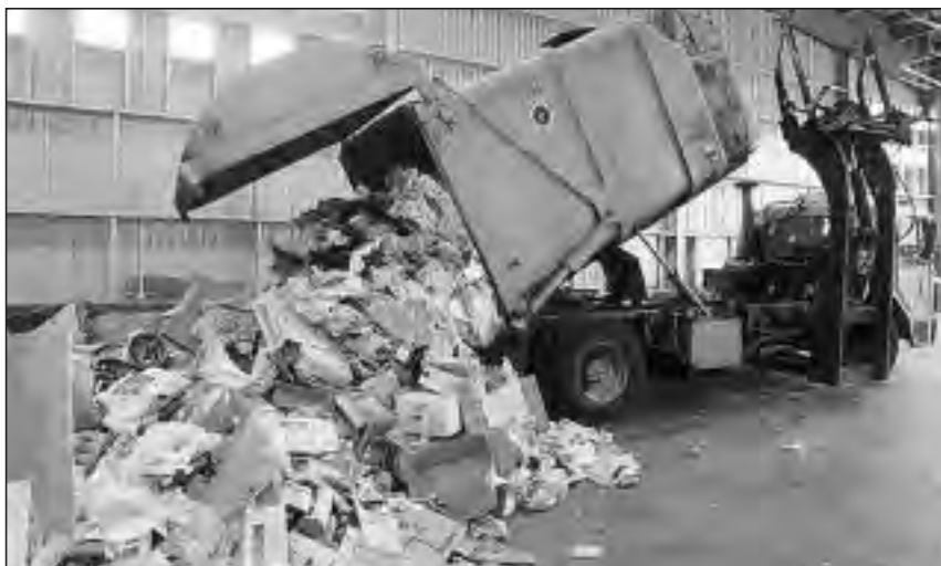
A collection vehicle dumps its load onto the tipping floor.
