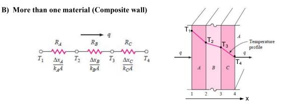
The heat flow must be the same through all sections, therefore,
