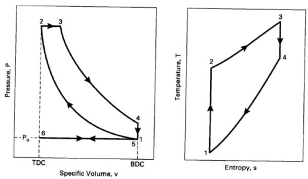
**Process** (6-1): Constant pressure intake of air at  $(P_o)$ . Intake valve open and exhaust valve is closed.
