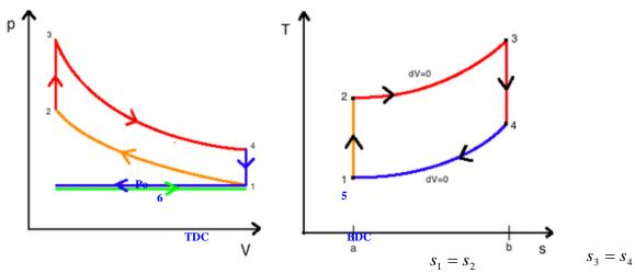
**Process** (6-1): Constant pressure intake of air at  $(P_o)$ . Intake valve open and exhaust valve is closed.
